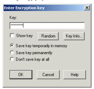
Enter encryption key or password required. Push button *Random* generates random encryption key (which can be seen by pressing *Show key* or *Key Info...*). You can optionally save the password/key temporarily in memory, where it will be stored until Stratesave program is quit, or store it permanently. See also chp. 8.14., "Where the passwords/encryption keys are stored".
